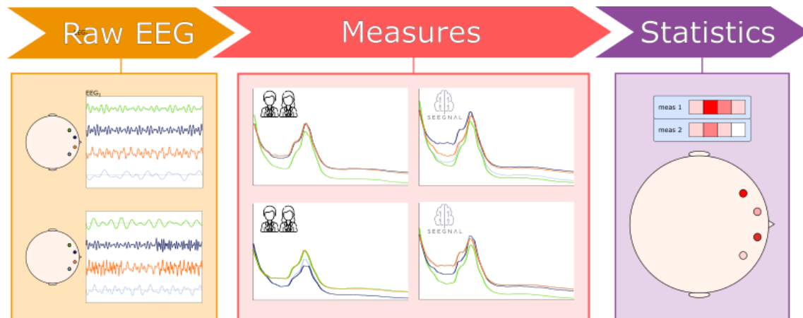
Figure 5. Pipeline to assess sEEGnal performance using the power spectrum. For the sake of clarity, this example is simplified by considering only two recordings, the frontal area, and one metric. The power spectra of frontal channels are estimated using the data obtained either by sEEGnal or the human EEG experts. The power spectra of each channel are compared using correlation and NRMSE, and the average is plot in head space for spatial visualization.
