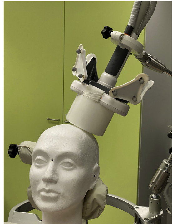
Figure 3. The stimulation coil with a 75-mm-high plastic block for sham stimulation.
