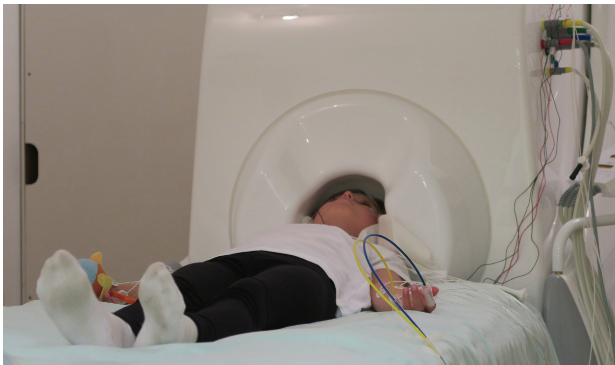
Fig. 2. A magnetoencephalography recording during the TASK condition. The subject is lying still on the bed with the subject's head in the dewar helmet. The thin plastic tubes (blue and yellow) are connected to the Somatosensory Stimulus Generator outside the magnetically shielded room and drive air pulses to plastic diaphragms gently fastened with skin tape to the subject's left index and little finger. The subject is holding a soft nonmagnetic toy in the right hand in order to respond to the tactile stimuli the subject feels on the little finger. (For interpretation of the references to colour in this figure legend, the reader is referred to the web version of this article.)
