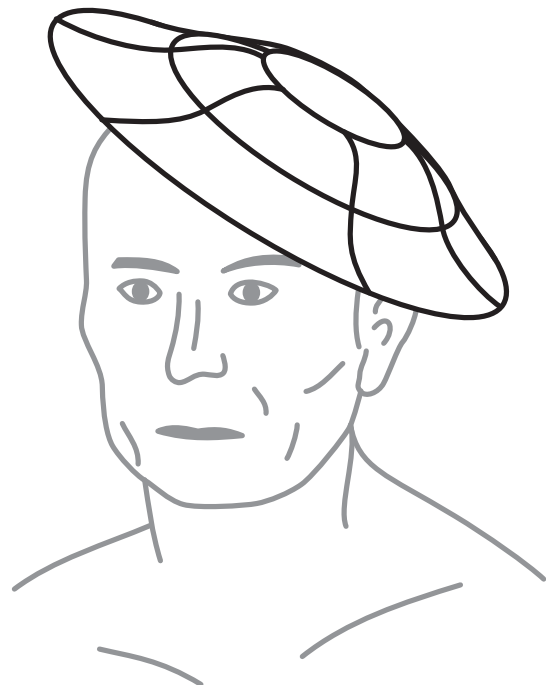
Fig. 1. An example of an overall coil shape with one surface with a flat central part and a curved exterior part.
